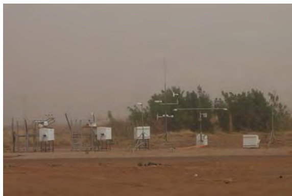
In March 2006, the ARM Mobile Facility and satellite instruments made the first simultaneous observations of a major dust storm from space and the ground, allowing researchers to test their understanding of how dust affects the radiant energy budget of the atmospheric column.
