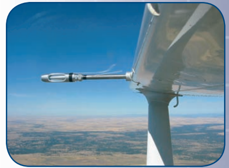
The Cessna aircraft's new, improved sampling probe design will provide much better measurements of larger particles.
