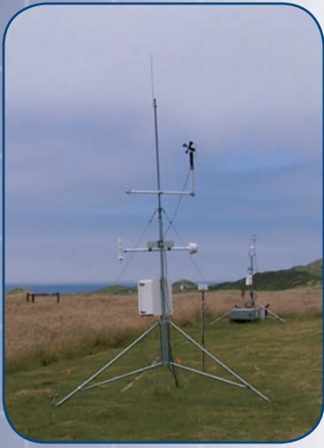
With the Pacific Ocean in the distance, a surface meteorology system collects wind, temperature, pressure, and humidity data as marine clouds drift over the field instruments at the AMF deployment site at Point Reyes National Seashore.
