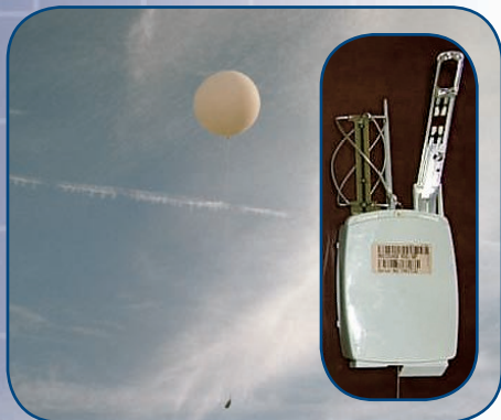
At the end of a string tied to the weather balloon, a small sensor package, called a radiosonde, contains the “brains” for measuring atmospheric temperature, pressure, and humidity.
