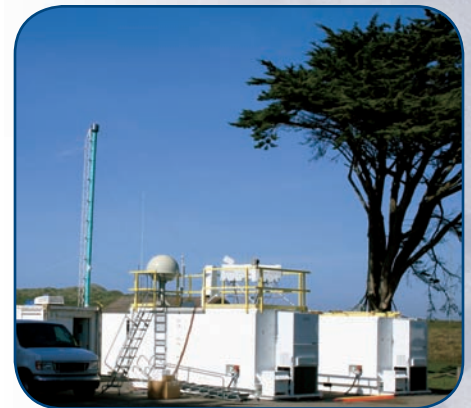
State-of-the-art active and passive remote sensors measured the detailed microphysical structure of marine stratus clouds at the AMF deployment site, about 1 mile from the ocean at Point Reyes National Seashore.
