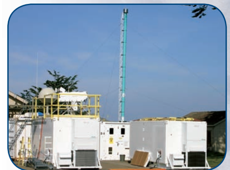
An aerosol observing system (green stack) was added to the baseline suite of AMF instruments after proving its value during a successful 6-month field campaign at Point Reyes National Seashore in California in 2005. In 2006, the AMF begins a yearlong deployment in West Africa.
