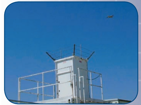
The Jetstream-31 made numerous passes over the Raman lidar at the SGP site during ALIVE. The Raman lidar is an active, ground-based laser remote sensing instrument that measures vertical profiles of water-vapor mixing ratio and several cloud- and aerosol-related quantities.
