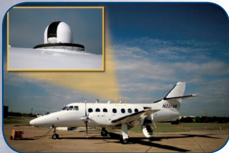
Outside the hangar in Ponca City, Oklahoma, the optical head of the AATS-14 (inset) can be seen as the white dome on the roof of the Jetstream-31 aircraft. The AATS-14 obtained extinction vertical profiles from spiral ascents and descents over the SGP site during ALIVE.
