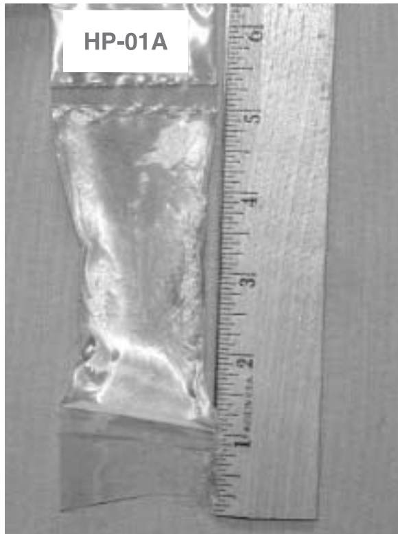
Figure 9. Passive-diffusion-bag sampler. (Photograph by Daniel J. Phelan, USGS, 2001.)
