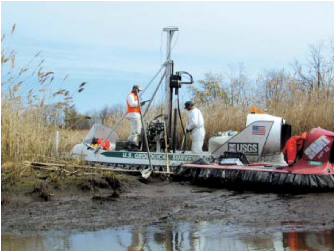
Figure 7b. The Hoverprobe and support hovercraft at site HP08, West Branch Canal Creek wetland, Aberdeen Proving Ground, Maryland.
