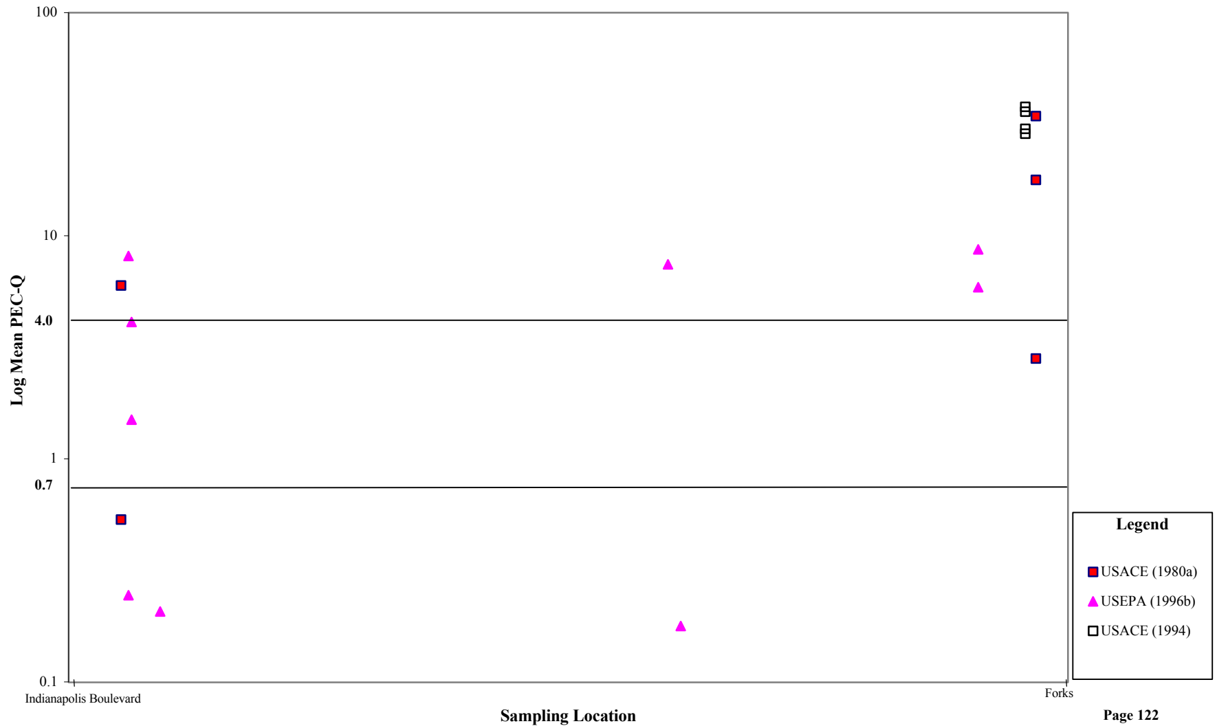
Figure 12.8b. Spatial distribution of mean PEC-Qs in sub-surface sediments within the Indianapolis Boulevard to Forks segment of the USC.
