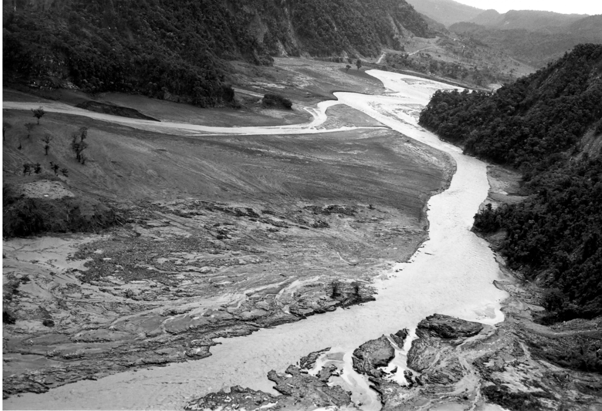
Fig. 3. Looking downstream at the confluence of the Malo River (flowing from the left) with the Coca River, northeastern Ecuador, following debris-flow activity induced by the 1987 Reventador earthquakes. A debris flow issuing from the Malo River during the night of 5 March 1987 formed a short-lived dam of the Coca River, resulting in deposition of ~15 m of sediment in the Coca channel (Nieto et al., 1991).
