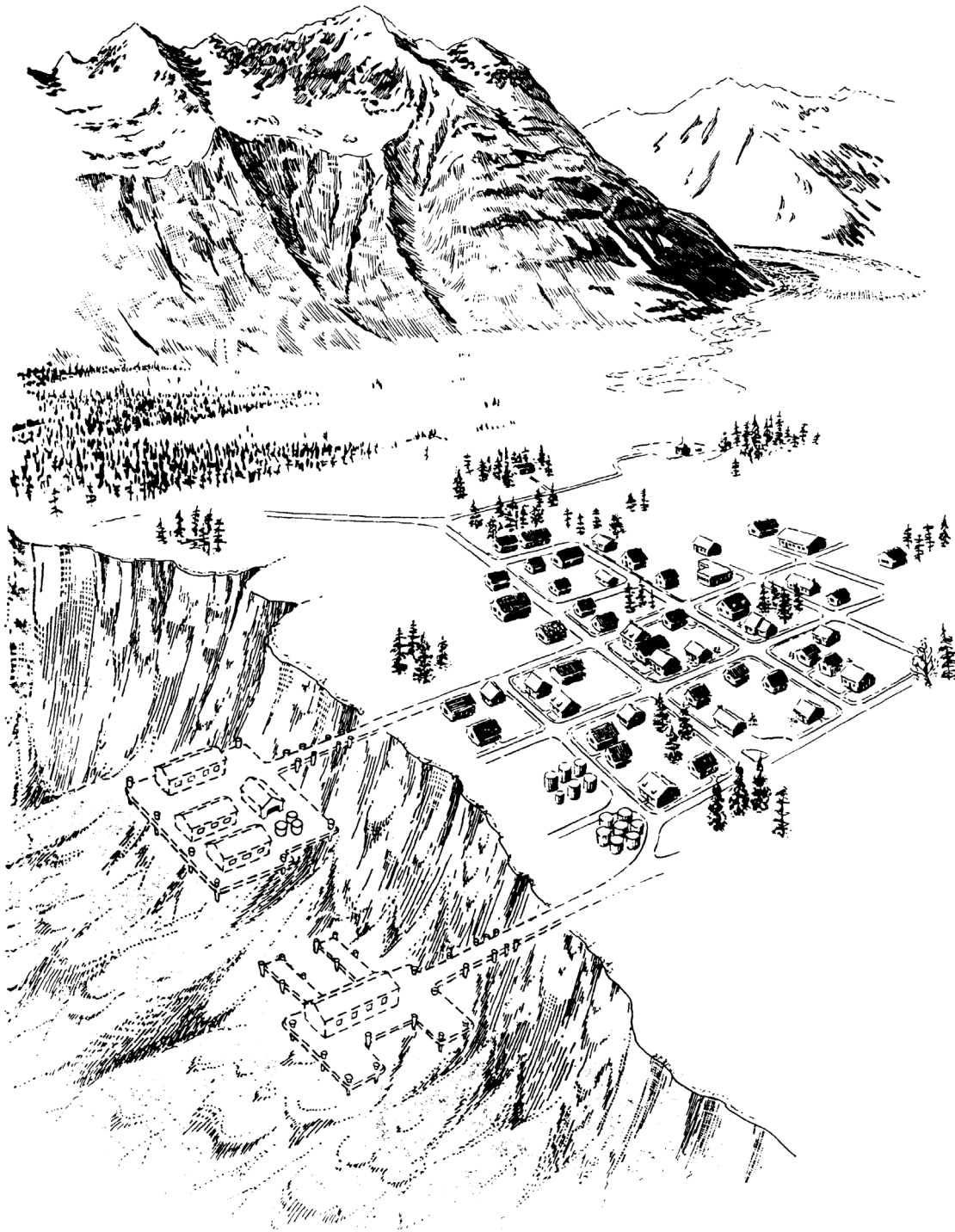
Fig. 10. Destruction of shoreline and port facilities at Valdez, Alaska, by a submarine landslide triggered by the March 1964 Alaska earthquake (Coulter and Migliaccio, 1966). Dashed lines indicate dock area destroyed by the slide. (Drawing by David Laneville, U.S. Geological Survey.)
