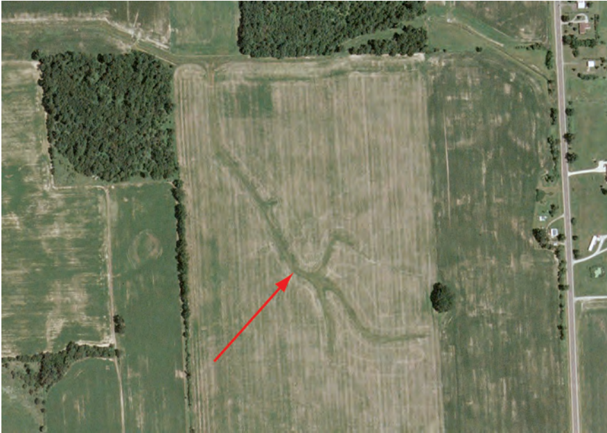
Figure 12. A true color aerial photograph shows a new drainage network (indicated by red arrow) and provides visual evidence of wetland loss. Lack of wetland vegetation, surface water or soil saturation further indicates that this wetland had been effectively drained.
