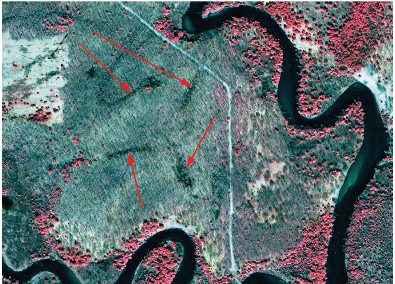
Figure 7. Early spring 2005 Ikonos satellite image of Michigan. Leaf-off condition made recognition of wetland features easier. These old oxbows or swales (indicated by red arrows) can be masked by heavy tree canopy later in the growing season. Image courtesy of Space Imaging Corp.
