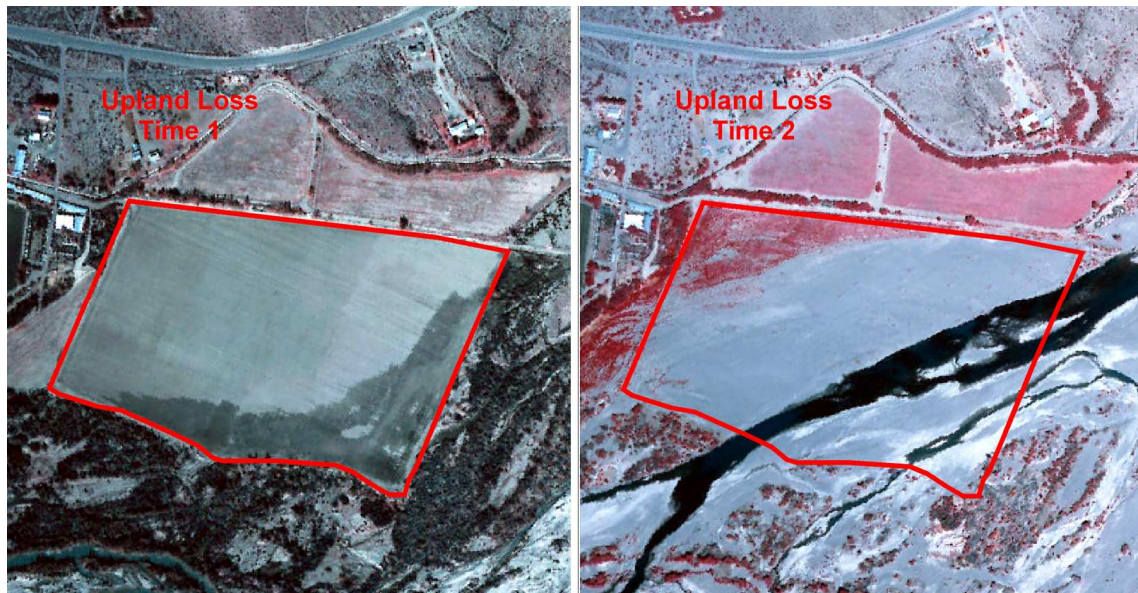
Figure 4. Upper Gila River floodplain, near Sanchez, AZ. Example of upland agriculture lost to channel change, as a result of the flood. CIR aerial photography, 1:15,840 scale, January 18, 2005 (left), May 19, 2005 (right).
