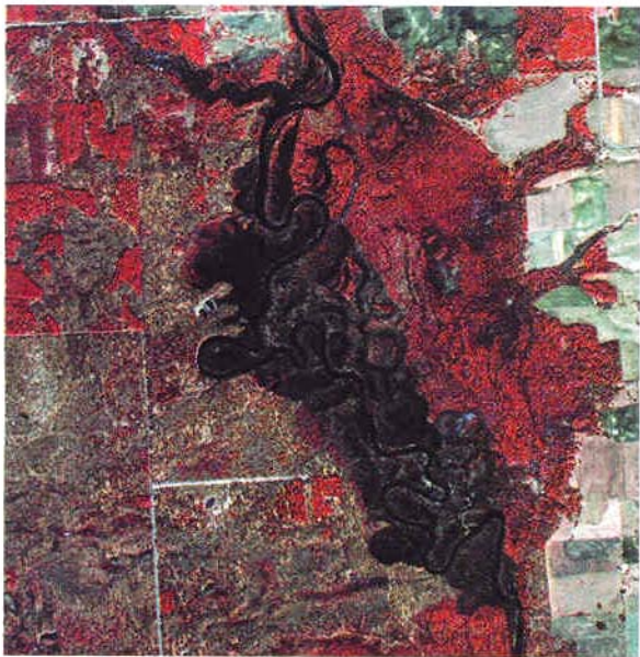
● Figure 2. An IKONOS image shows a large forested wetland complex in Wisconsin on early spring imagery. Darker tones along the river are primarily deciduous forested wetlands; red tones are evergreen upland forest.
