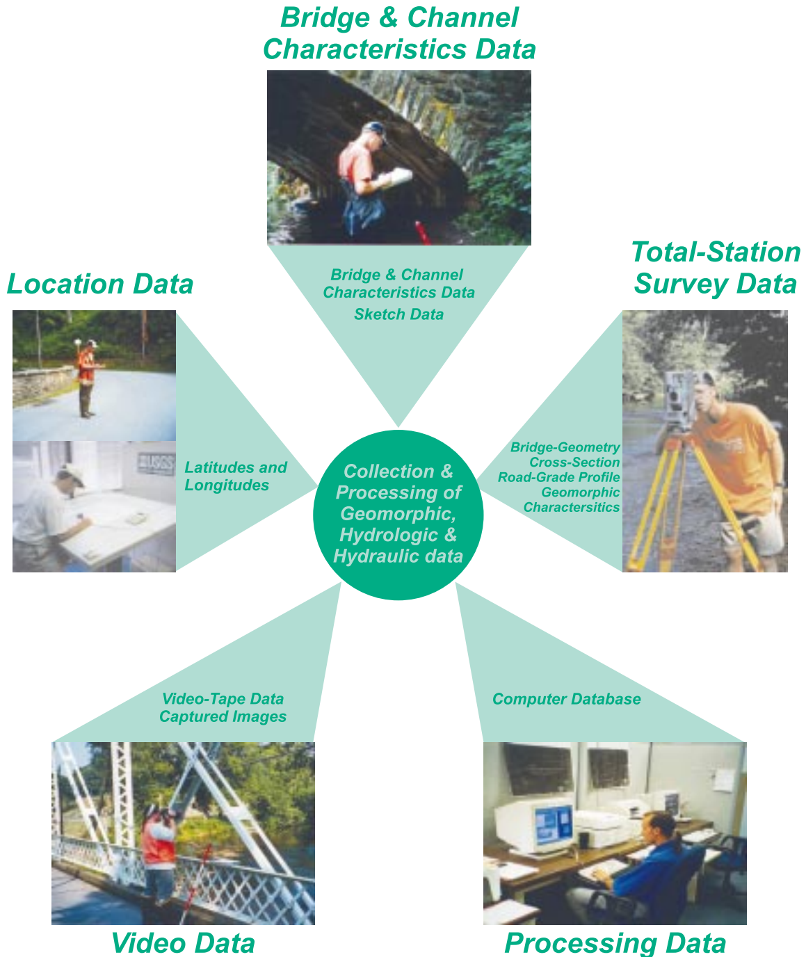
Figure 1. Collection and processing of geomorphic, hydrologic, and hydraulic data for assessment of scour at bridges.
