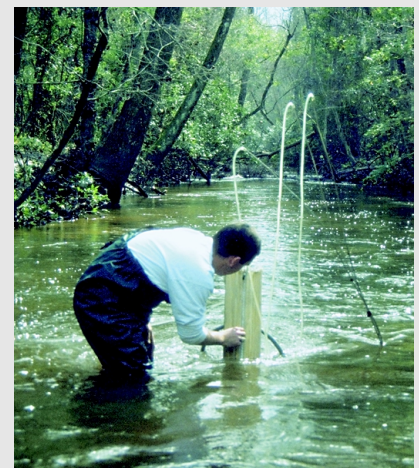
Water levels were measured simultaneously in Cow Castle Creek and at multiple depths in the aquifer below the creek. Under most streamflow conditions, water from the aquifer was moving upward into the creek.
