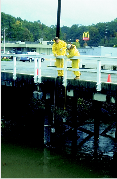
Stormwater samples for volatile organic compounds were collected by using special samplers developed for the NAWQA Program.
