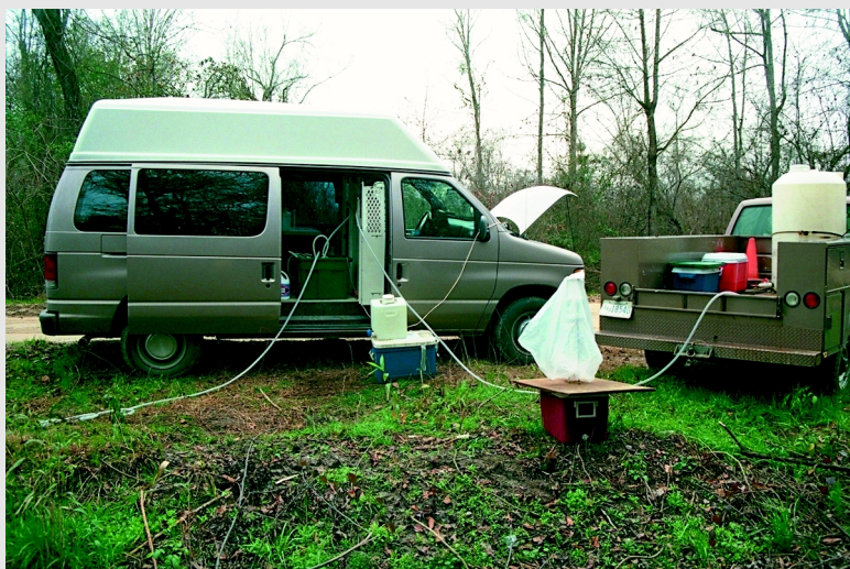
Ground-water samples are pumped directly into a mobile laboratory for processing samples and conducting field analyses.
