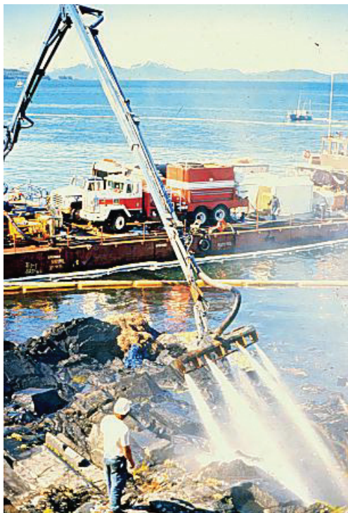
Omni-boom, with worker supervision, blasts oil coated rocks in an attempt to clean gross oil contamination from beach, LaTouche Island. Photo courtesy of the Exxon Valdez Oil Spill Trustee Council.
