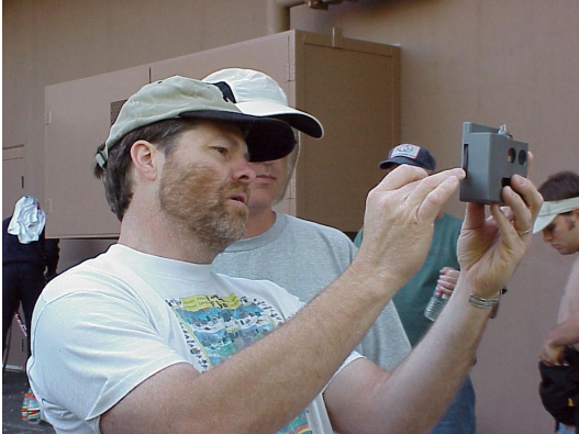
Paul Lander of the Boulder Water Board, one of the institute participants, checks a field meter for dissolved metals in a water sample.
