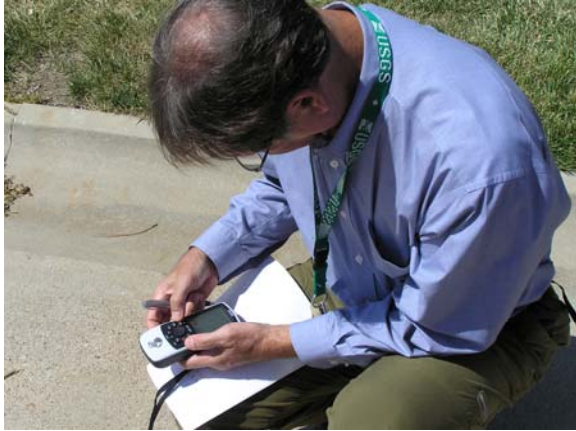
Collecting GPS coordinates and recording field data. We used the free Minnesota DNR Garmin program to bring the points to our ArcGIS map document.
