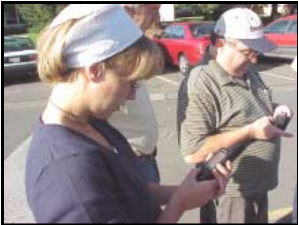
GPS coordinate collection brings in a host of considerations important to GIS work, particularly those of coordinate systems and datum shifts. We later brought the coordinates into ArcGIS, overlaying them on top of a USGS DOQ and a DRG.
