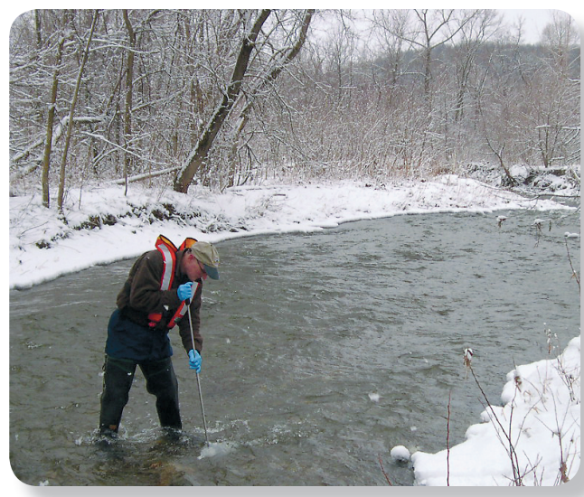
A USGS scientist wades a river in Chittenden County, Vermont, to collect a water-quality sample.
