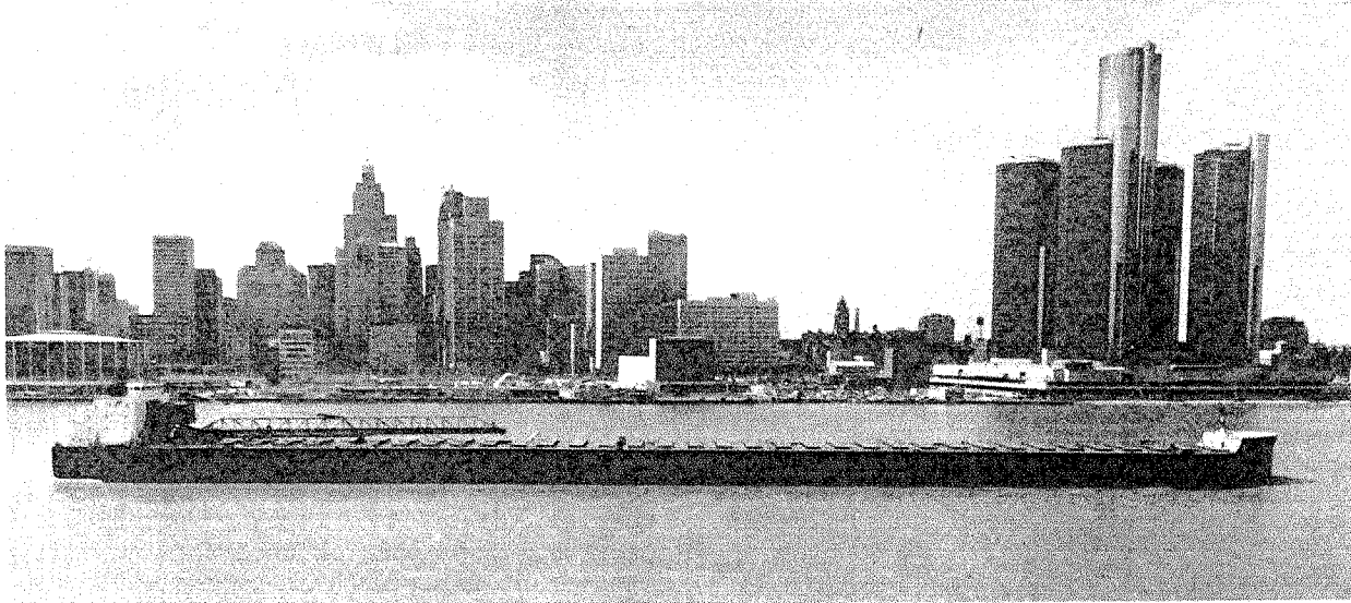
Figure 4. Large self-unloading lake carriers, such as the Mesabi Miner shown here passing the City of Detroit, Michigan, carry bulk cargoes of iron ore, coal, limestone, and grain (Photo provided by Albert G. Ballert).
