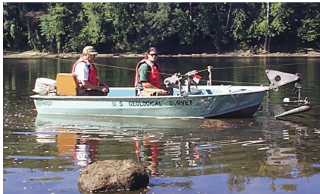
Monitoring the health of the Nation's water supply. Measuring river flow along a tag line.
