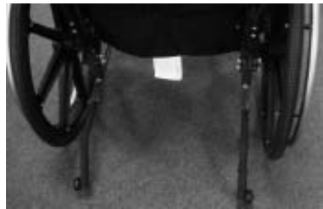
Figure 6.48. Anti-tip wheels also contribute to maneuverability.
