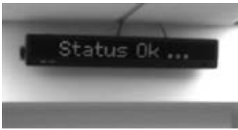
Figure 5.69. The display indicates an OK status and, when necessary, provides other indications of refrigerator problems.
