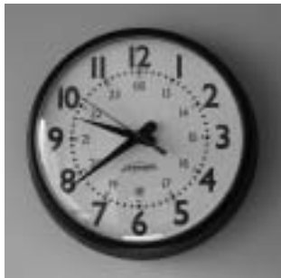
Figure 8.38. This clock is part of a system. One receiver communicates wirelessly with each clock in the facility.
