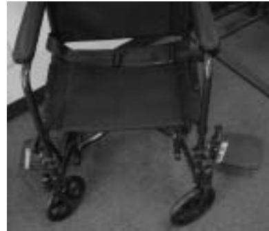
Figure 3.31. The footplate can be released and moved to the side.
