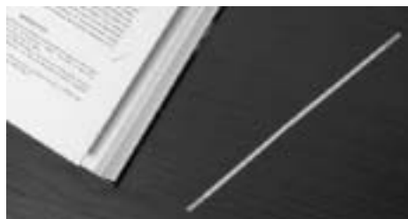
Figure 6.51. A narrow strip of magnetic material, accompanied by exit door sensors, helps deter library thefts.
