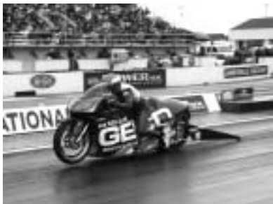
Figure 6.49. The wheelie bar helps the driver maintain control of the motorcycle. Photo by Matt Polito. Used with permission.
