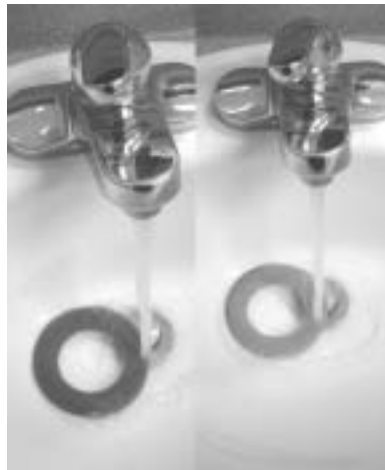
Figure 5.3. These plastic rings change color at 40 °C.
