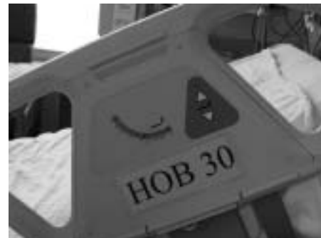
Figure 6.34. In addition to the gauge on the railing, the label is mounted to indicate to nurses whether or not the bed is situated at the correct angle.
