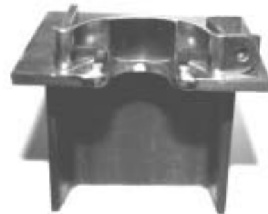
Figure 4.8B. A fuel filter clamp loaded in a work fixture. Photos from Erlandson et al. 10 © 1998 IEEE. Used with permission.
