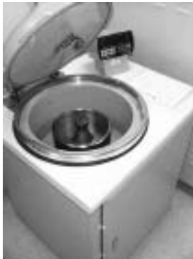
Figure 6.33. The cover on this centrifuge cannot be opened until rotation approaches zero. Copyright © 2006 Tandex Test Labs, Inc. Used with permission.
