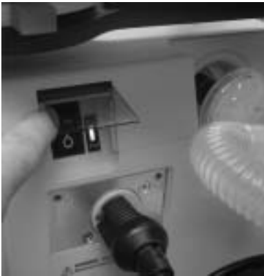
Figure 5.62. The switch on the back of this machine prevents inadvertent bumping.
