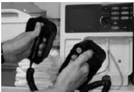
Figure 6.19. This defibrillator requires two-handed operation.
