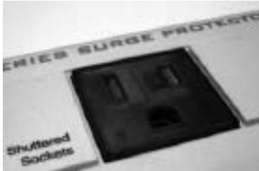
Figure 8.14. Insertion in the outlet of this surge protector is blocked to plugs with less than two prongs.
