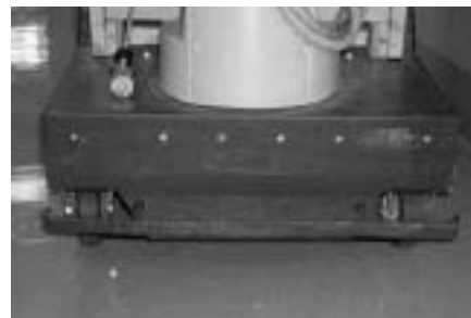
Figure 6.14. A front bumper switch stops the machine upon contact.
