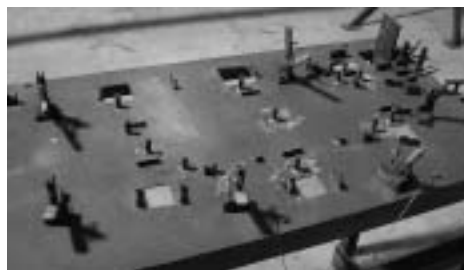
Figure 6.30. A fixture for holding parts during fabrication. Photo by Jon Timlin. Used with permission.
