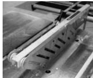
Figure 4.4B. Close up photo of a blade guard. SawStop is an intriguing, alternative safety device for table saws that is very effective. Workers may not even know about it until it saves their fingers. (Video of SawStop’s function can be seen at www.mistakeproofing.com .)
