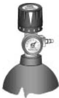
Figure 5.9. Regulator dial indicates the amount of oxygen delivered in liters.
