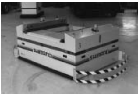
Figure 6.15. A guided vehicle system stops this robot when contact is made. Image from Frog Navigation Systems. www.frog.nl . Used with permission.
