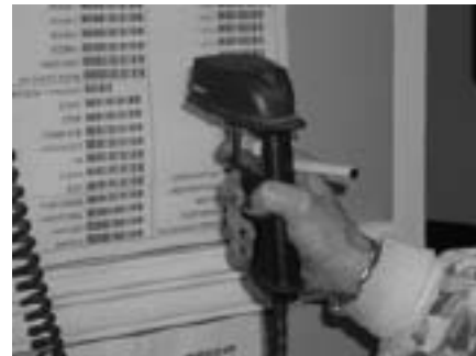
Figure 8.3. The bar codes are laid out on the wall in close proximity, a design that is inattentive to human factors considerations.
