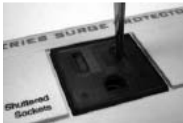
Figure 8.15B. The shutter is designed to prohibit insertion in either slot.
