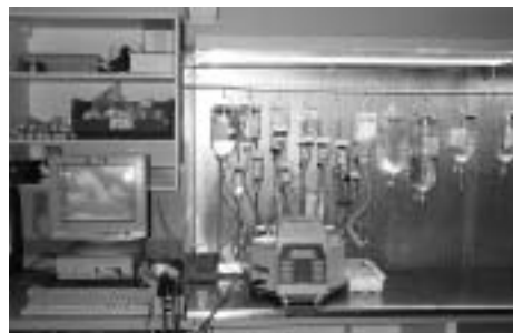
Figure 8.4. Software ensures that this automixer optimizes proportions of ingredients for TPN solutions.
