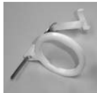
Figure 5.50. The hoop in this dental x-ray film holder provides a target for the technician.
