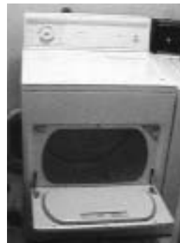
Figure 6.10. The clothes dryer stops operating when the door is opened.
