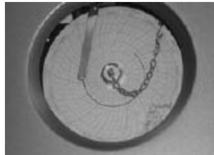
Figure 5.68. Blood bank refrigerators monitor temperature and produce chart recordings and digital visual readings.
