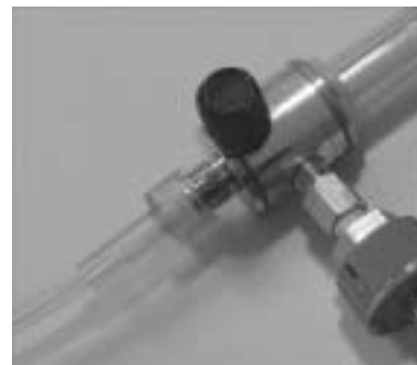
Figure 5.13B. Tubing attached to a regulator without a nozzle.
