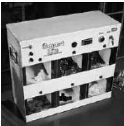
Figure 4.5. A pick-to-light bin system.
