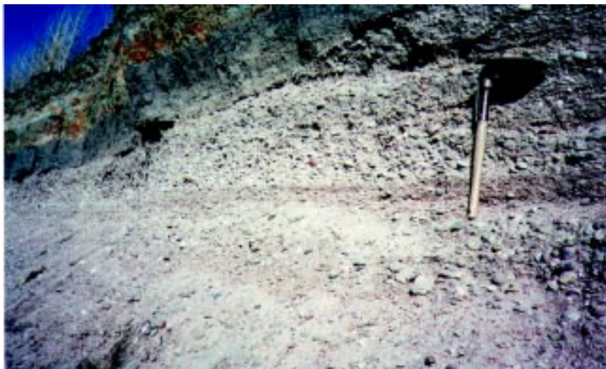
Figure 8. —Photograph showing soil and overbank sediment in erosional contact with upper gravel unit, east side Mann Lake pit. Gravel is a clast-supported pebble deposit, moderately well-sorted, with sand occupying interstices.
