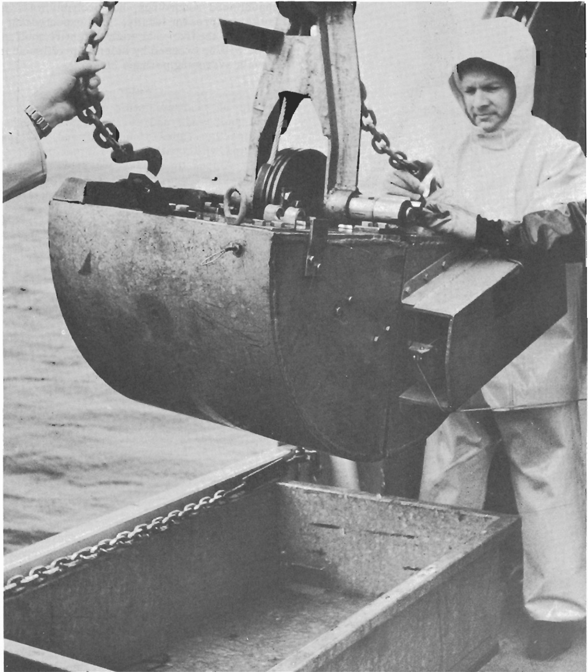
Figure 2.-Large Campbell grab made by Logan Smith of Wilmington, California
