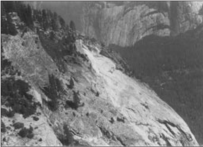
Figure 3. Rock-fall release (center) and steeply inclined ramp along which blocks slid from left to right before beginning free fall beyond right edge of photograph. Yosemite Valley and Royal Arches are in background. Approximate length of ramp from release (center) to lower right edge of photo is 235 m. (Photograph by Doug Roe, National Park Service.)
