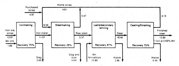
Recovery with respect to ferromanganese additions is assumed to be 82 percent, while complete recovery of Mn is assumed for raw steel
