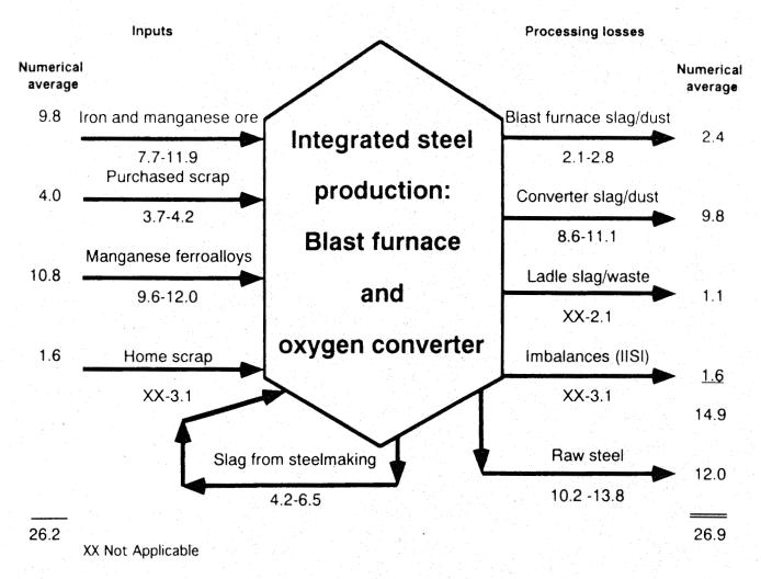
Figure 8.—Composite of manganese balances for integrated steel production in pounds of manganese per ton of raw steel. Based on data of OTA (reference 2, 1985), IISI (reference 8, 1980), and NMAB (reference 1, 1976).
