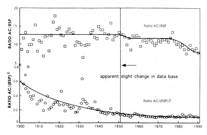
Figure 13.—Relationships between manganese apparent consumption (AC) and raw steel production (RSP), 1901-90.
