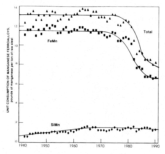
Figure A-4.—Time trends in unit consumption of manganese ferroalloys in U.S. steelmaking, 1942-90.
