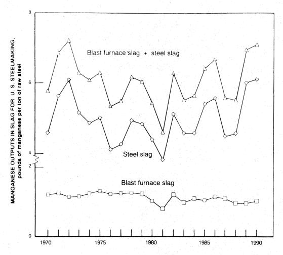
Figure A-6.-Manganese outputs in slag for U.S. steelmaking, 1970-90.
