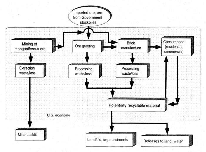
Figure 11.—Flow diagram for manganese use in brick coloring.
