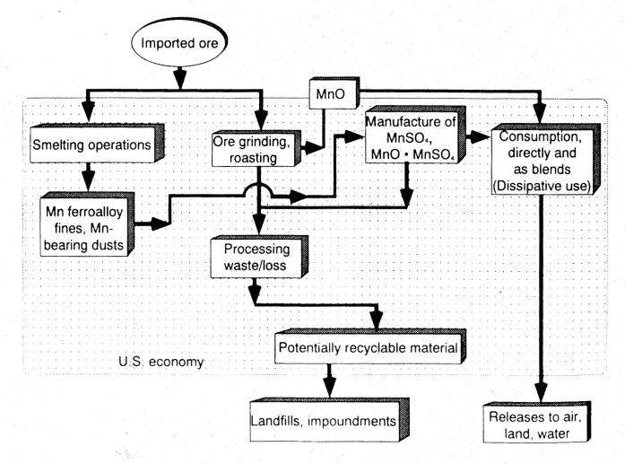
Figure 12.—Flow diagram for manganese use in animal feed and plant fertilizer.
