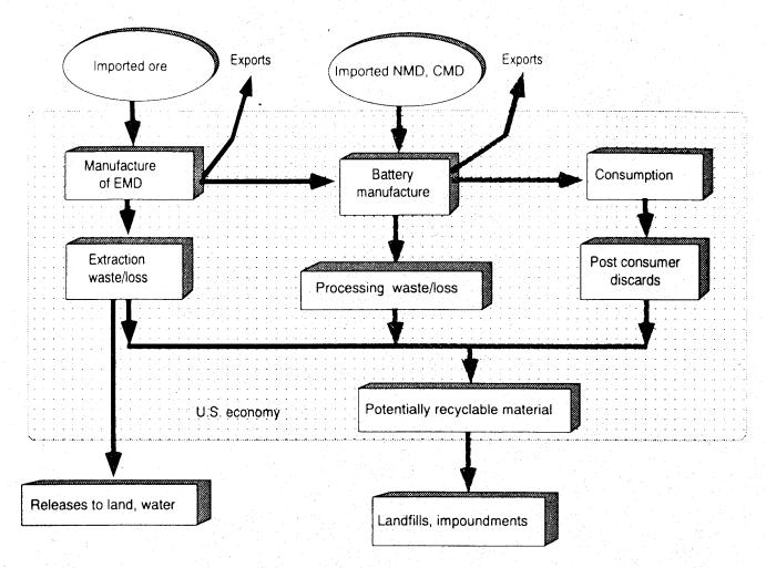
Full diagram applies to electrolytic manganese dioxide (EMD).
