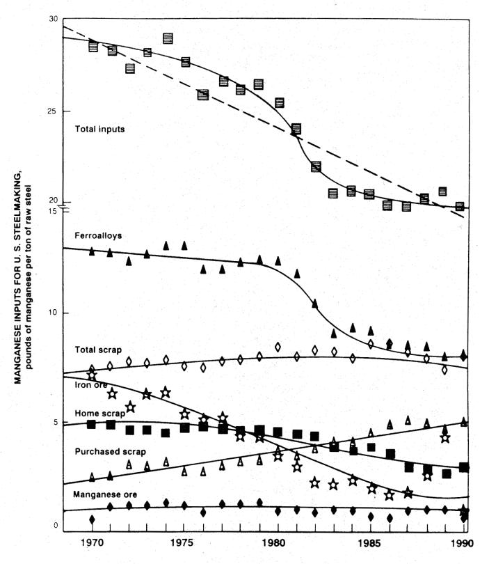
Figure A-5.—Manganese inputs for U.S. steelmaking, 1970-90.
