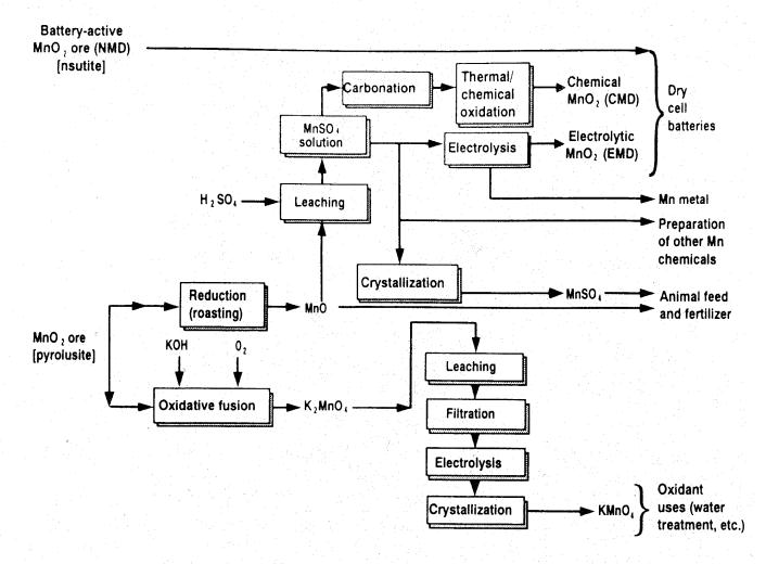
Figure 6.—Simplified diagram of processing and uses for key manganese chemicals.
