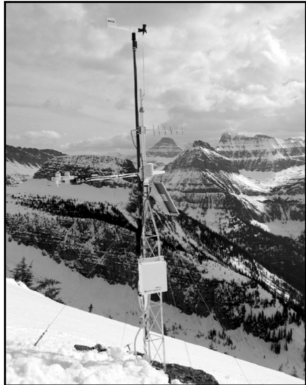
Figure 10: Garden Wall weather station (2240m) installed December 2003 adjacent to the Haystack Creek avalanche paths.
