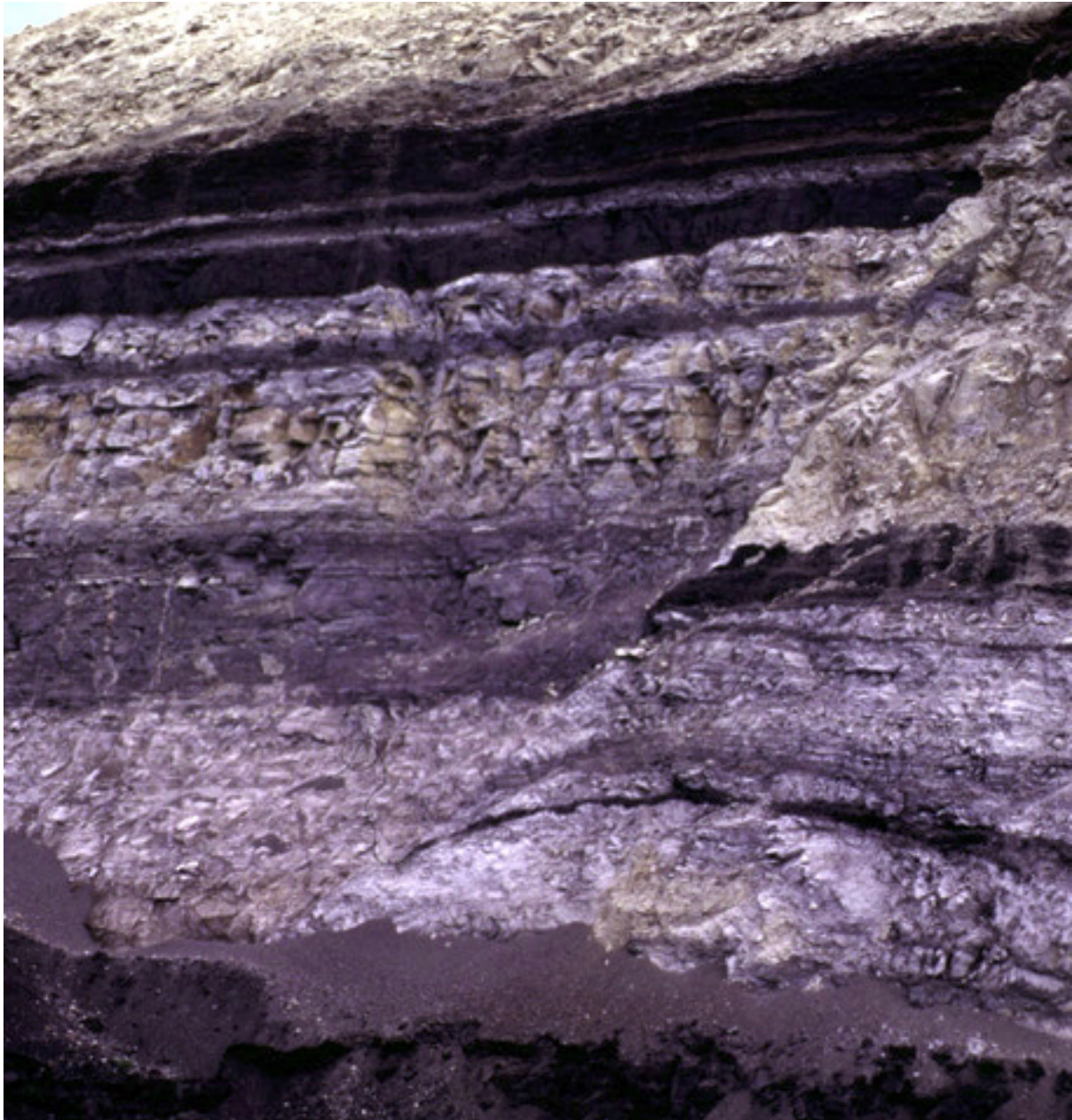
Figure HF-7. Coal (upper part of picture) with siltstone and mudstone partings in the Medicine Bow mine. Note normal fault on the right side of the picture. Photograph by R.M. Flores.
