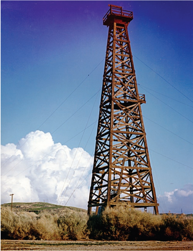
Figure 3.14. A wooden derrick, site unknown, typical of those used during much of the early oil exploration of the San Joaquin Valley. Photograph courtesy of Don Arnot, West Kern Oil Museum.
