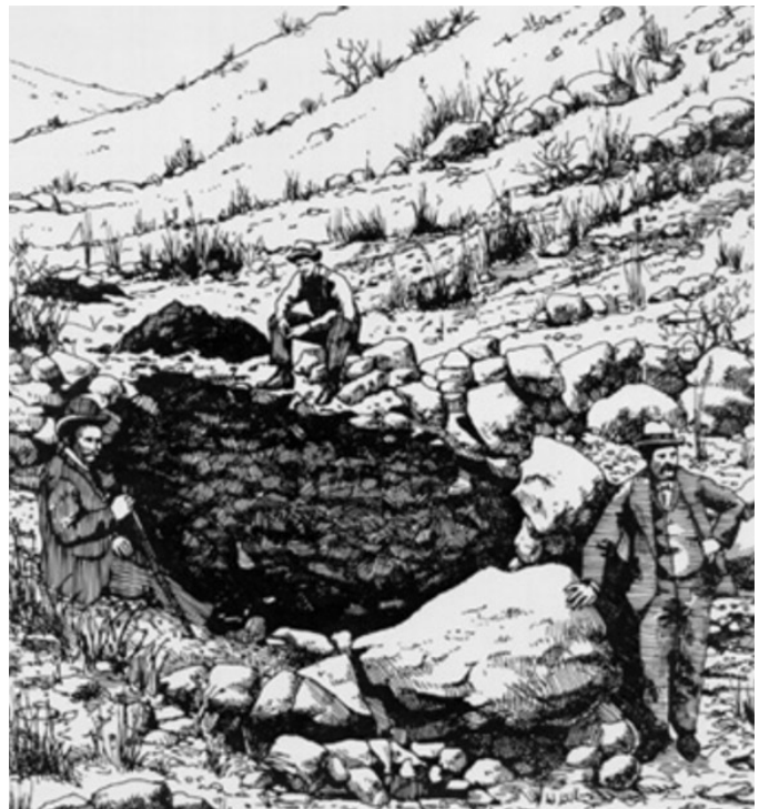
Figure 3.8. Asphalt was first mined by digging open pits where seeps occurred, in this case near McKittrick, in Kern County. Drawing by J. Spriggs, from Onshore Oil and Gas Seeps in California ( http://seeps.wr.usgs.gov/seeps/index.html ).
