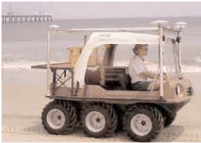
The SWASH (Surveying Wide Area of Shorelines) system, developed by the USGS for accurate measurements of shoreline position using recent advances in the Global Positioning System (GPS). See p. 15.
