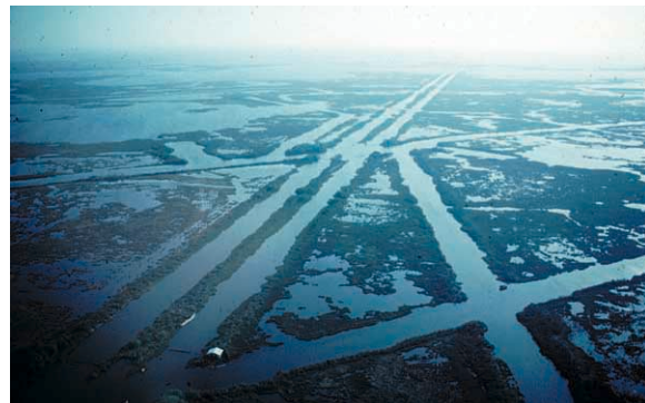
Figure 10. Air photograph of canals dredged in Louisiana's wetlands for navigation and energy development; these canals have accelerated wetland loss over the past 50 years. USGS photograph taken in about 1985.
