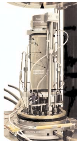
Figure 32. Part of the GHASTLI system built by the USGS to study gas hydrates. USGS photograph.
