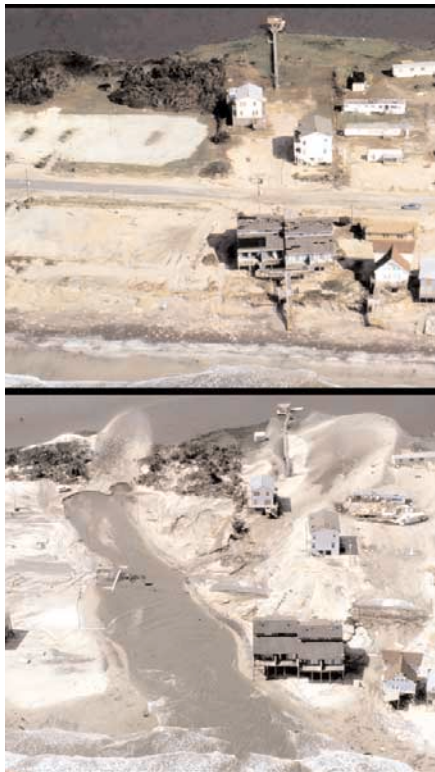
Figure 19. Topsail Island, a developed barrier island off North Carolina: above, the area on July 17, 1996, post-Hurricane Bertha/pre-Hurricane Fran; below, the area on September 7, 1996, post-Hurricane Fran, showing the dramatic effects of storm surge overwash. USGS photographs.
