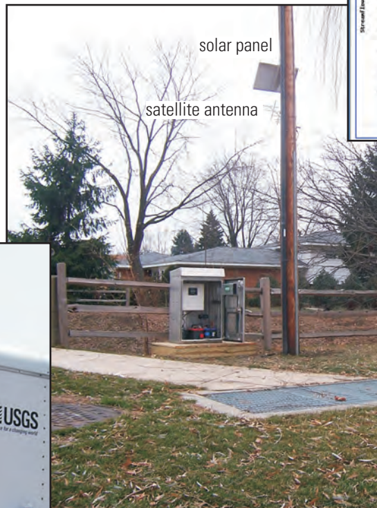
MWRDGC drop shaft DS-6 and USGS instrument enclosure at Mt. Prospect, Illinois. Note the solar panel and satellite antenna located above enclosure on the pole.
