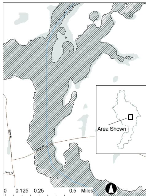
Figure 2. Comparison of observed and simulated inundation using NEXRAD rainfall at two sub-basins Lake Run tributary to Blackberry Creek, Kane County. the observed inundation image was developed from video taken in the afternoon of July 18, 1996, and presented as hatched areas. The inundation obtained from simulated peak discharges are presented in gray areas.
