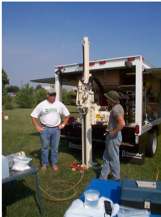
Collecting ground-water samples with the Geoprobe™ in Dover, Delaware.
