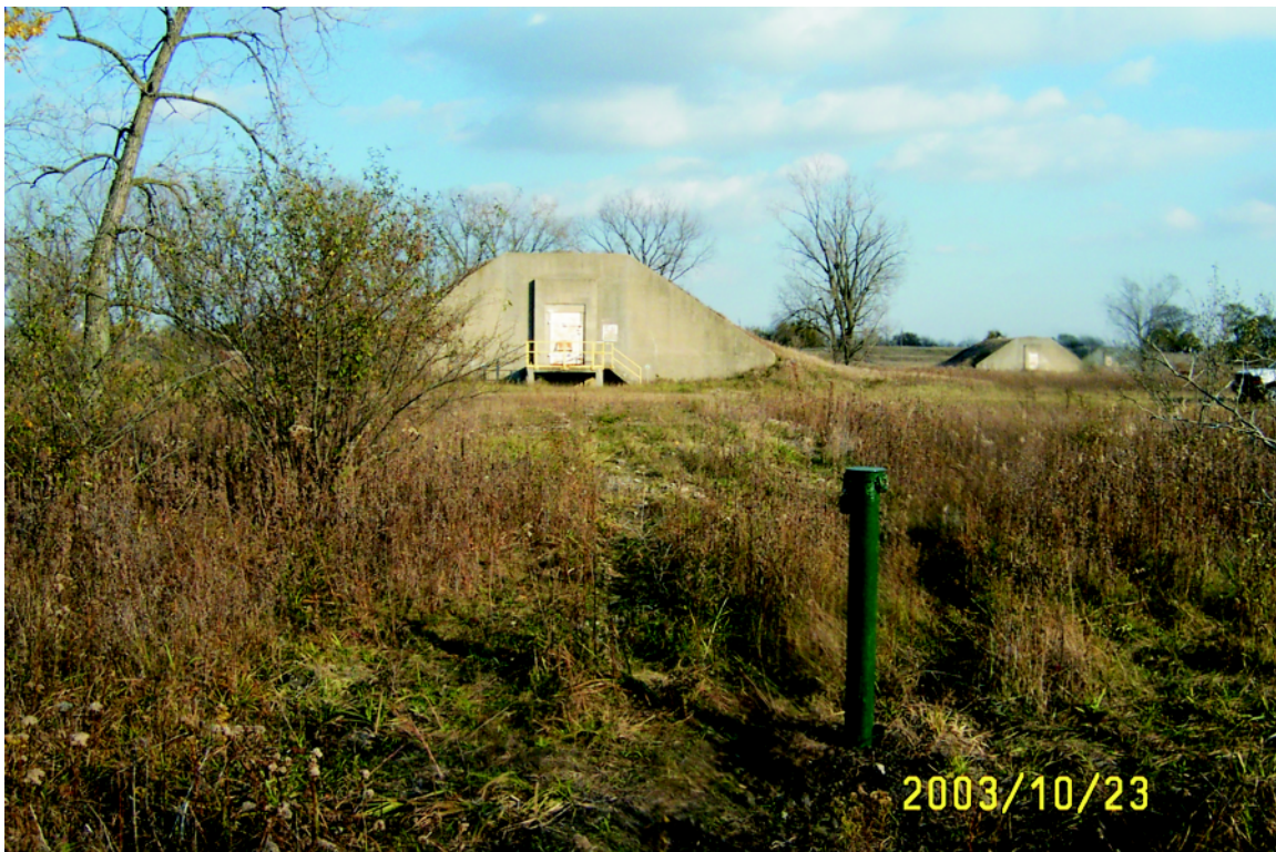
Figure 3. Piezometer installed in an outwash-plain wetland adjacent to a munitions bunker field at Midewin. Photograph by Patrick C. Mills.
