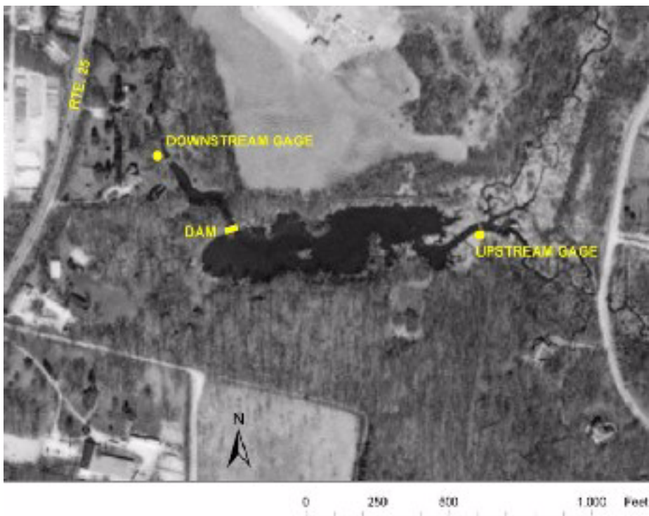
Figure 1. Location of two USGS gages in relation to the dam on Brewster Creek near St. Charles, Illinois.
