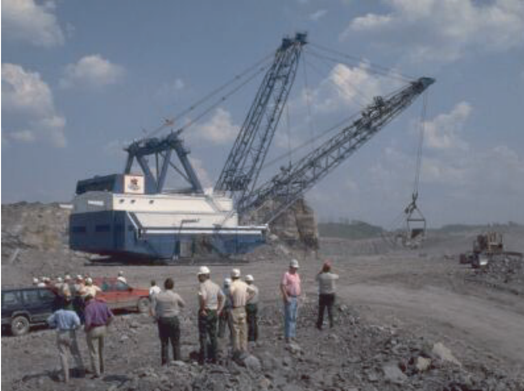
Figure 15. Photograph showing mountain-top removal mining operation in West Virginia. In mountain-top removal surface mines, large amounts of overburden are removed with draglines and dozers to expose multiple benches of low-sulfur coal. The overburden is deposited in heads of adjacent stream valleys. When mining is completed, some of the overburden is returned to the ridge tops to reconstruct original topographic contours. Photograph by West Virginia Geological and Economic Survey.
