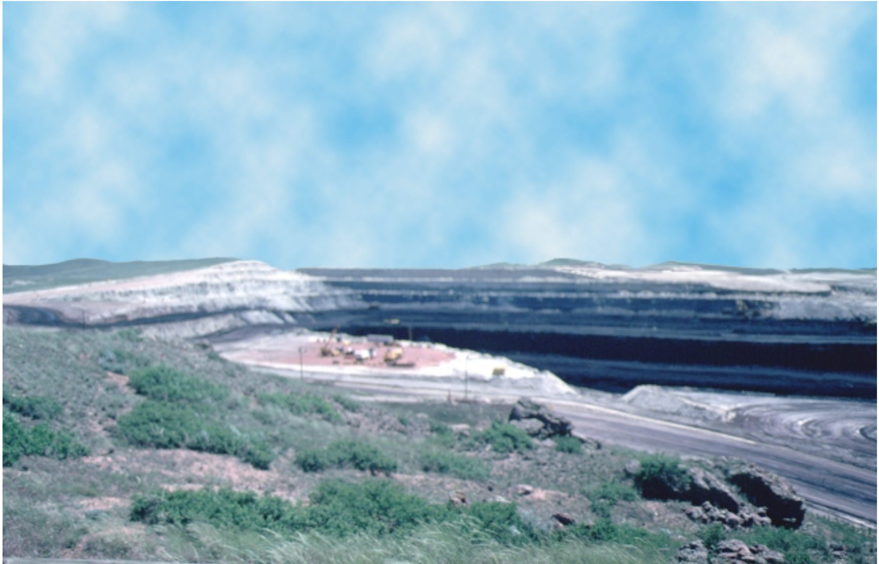
Figure PH-2. Coal beds of the Wyodak–Anderson coal zone and overlying carbonaceous shale, mudstone, siltstone, and sandstone in the highwall of the Big Horn mine. Photograph by R.M. Flores.
