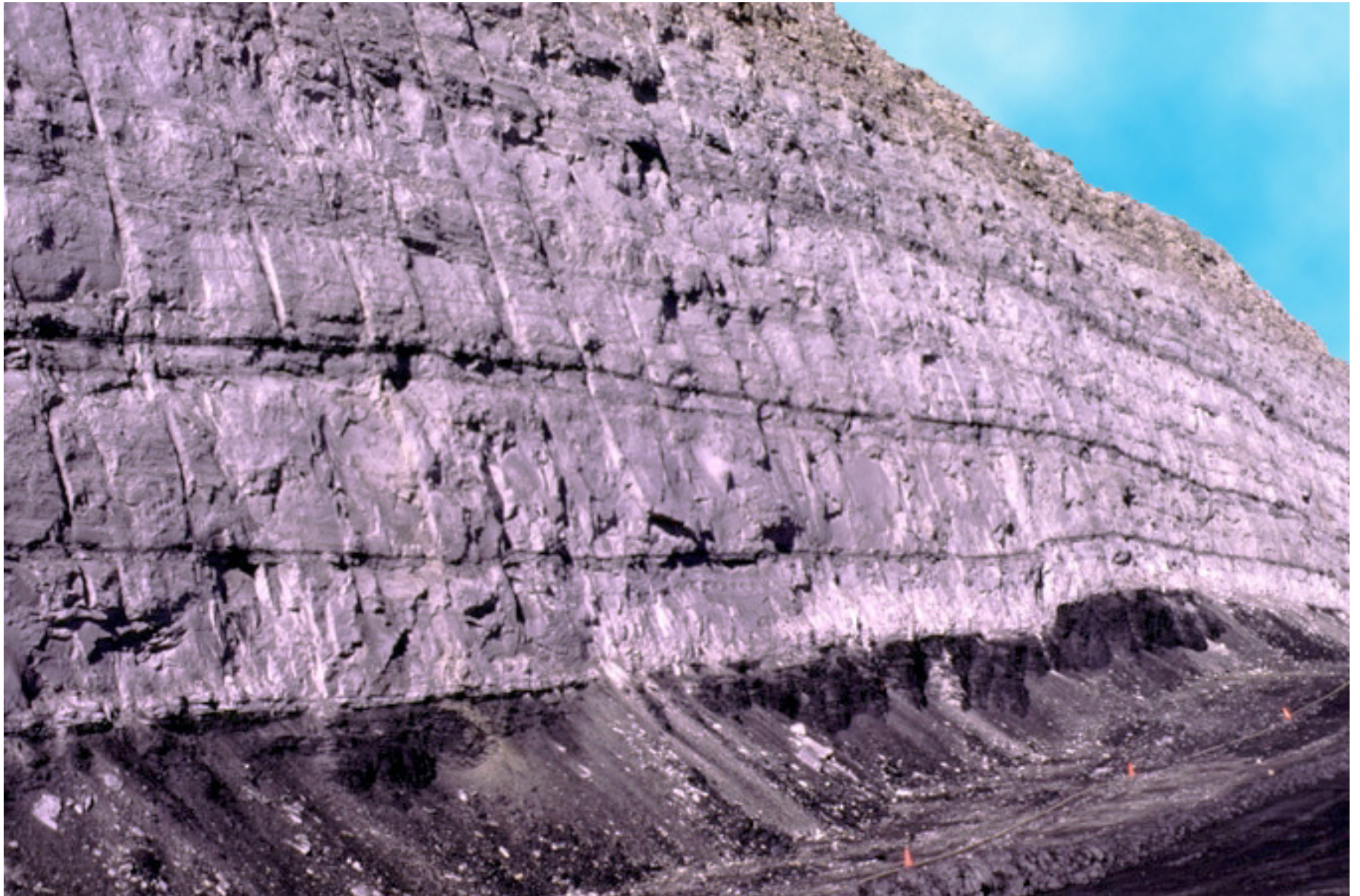
Figure GF-6. Fining-upward, stacked sandstone thinning from right to the left of the picture into thin-bedded silty sandstone, siltstone, and mudstone above the Deadman coal zone in the Jim Bridger mine. Photograph by R.M. Flores.
