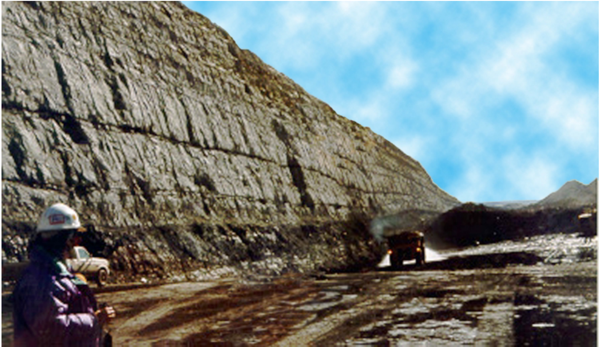
Figure GF-4. Stacked sandstone bounded by silty sandstone, siltstone, and mudstone above the Deadman coal zone in the Jim Bridger mine. Photograph by R.M. Flores.
