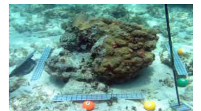
Coral surface area is critical to the sustainability of the coral reef community. Scales and billiard balls provide references for generation of 3-D models to determine surface area of live and dead coral.
