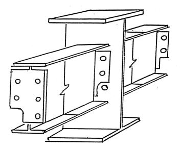
Clipped end connections are connection material on the end of a structural member which has a notch at the bottom and/or top to allow the bolt(s) of the first member placed on the opposite side of the central member to remain in place. The notch(es)
