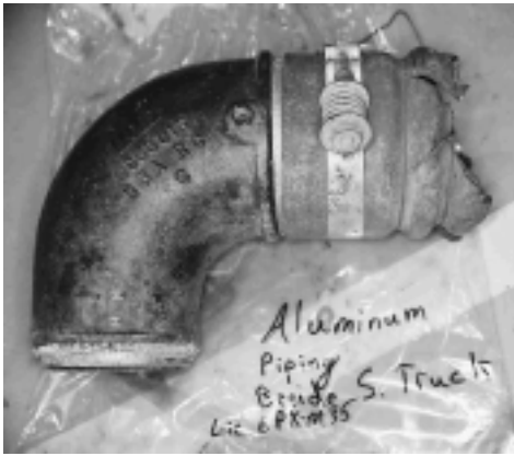
Figure 15. South truck diesel engine turbocharger discharge elbow.
