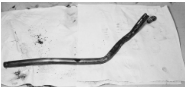
Figure 17. Bent exhaust valve pushtube, south truck diesel engine combustion chamber #2.
