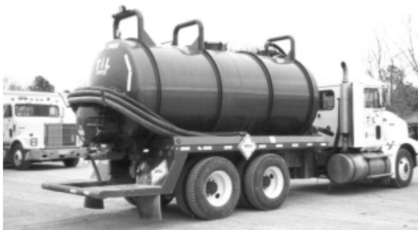
Figure 1. Typical vacuum truck used to haul oilfield waste liquids.
