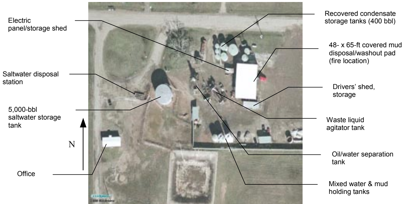
Figure 5. BLSR facility layout.
