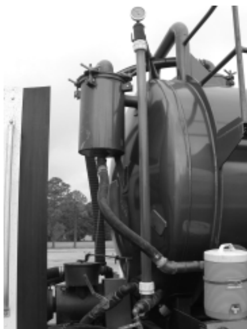
Figure 4. Typical vacuum truck tank sight gauge.
