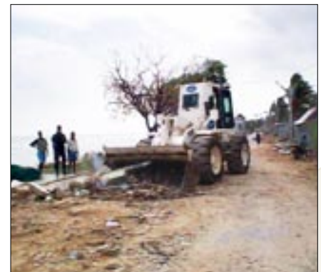
HALO Trust using a Volvo Front End Loader, armored and modified by them, to clear tsunami debris near Jaffria, Sri Lanka, shortly after the December '04 disaster.
