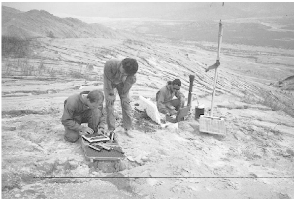
USGS and Filipino scientists verify operation of a mudflow-detection at Mount Pinatubo.
