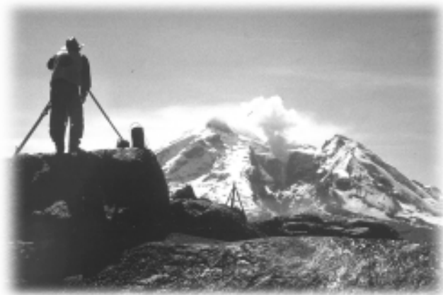
USGS scientist uses a theodolite to measure the volcano dome at Redoubt Volcano, Alaska (photo by USGS).
