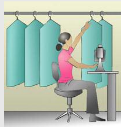
Fig. 1 Reaching overhead to pick up fabric can cause stress on the arms, neck, and shoulders.
