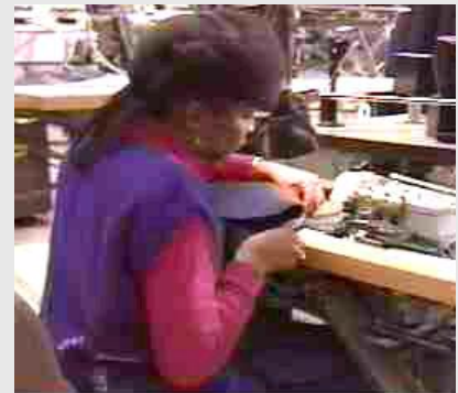
Fig. 1 Table too high, causing worker's left elbow to be raised.
