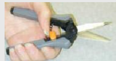
Fig. 2 Ergonomic snippers that spring back without operator force and minimize contact stress.
