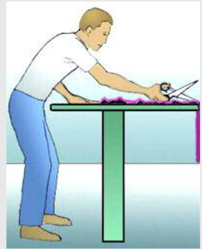
Fig. 1 Extended reach and bending over table causes ergonomic stress on back, shoulders, and arms.
