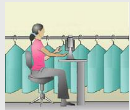
Fig. 5 Lowering the clothing rack can minimize overhead reach.
