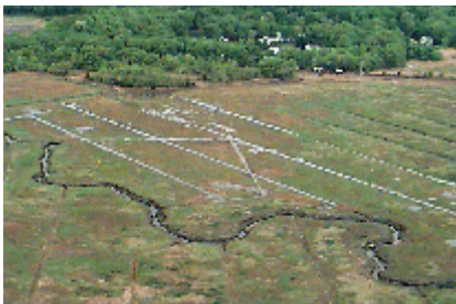
An aerial picture of the East River Marsh after the marsh restoration. Note that the old drainage ditches now hold water between high tides rather than draining the marsh.
