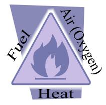
In an underground coal mine, the fuel for a fire or an explosion can be an explosive mixture of flammable gas, a sufficient concentration of coal dust, or a combination of both. The heat to ignite the combustible mixture can come from sparks, electrical arcs, detonation of explosives, etc. Oxygen sufficient to support combustion is generally present throughout unsealed areas.
