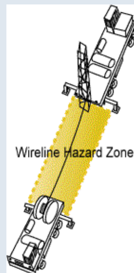
Fig. 2. Wireline hazard zone
