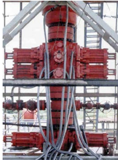
Fig. 1. Blowout preventer stack (BOP)
