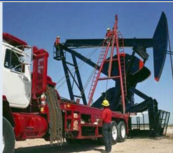
Fig. 2. Servicing horsehead and bridle
