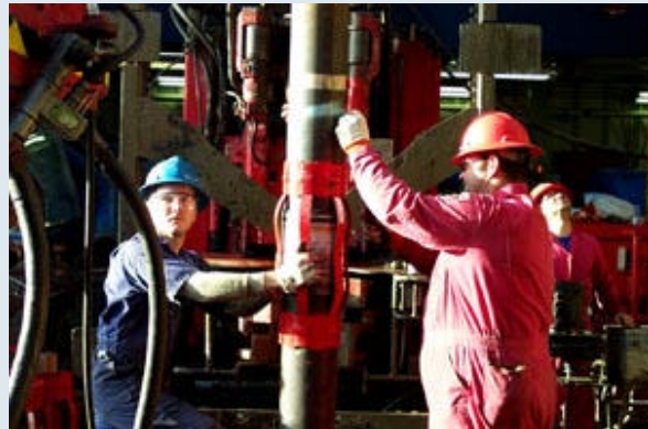
Fig. 7. Installing casing centralizer
