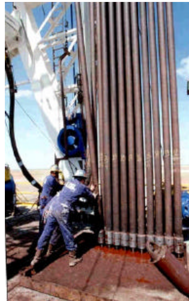
Fig. 1. Setting back a stand of drill pipe
