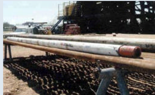
Fig. 15. Tubulars on pipe racks
