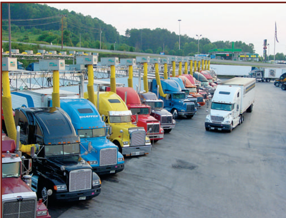
The Petro Travel Center in Knoxville, TN provides advanced truck stop electrification, limiting emissions.
