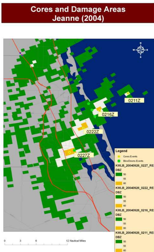
Fig. 14 Temporal composite of base reflectivity data from the Melbourne WSR-88D between 0211 and 0227 UTC 26 Sept 2004 (reflectivity below 50 dBZ removed). Note the core of the high reflectivity cell moving from offshore at 0211 UTC to nearly 10 km inland by 0227 UTC. Along the track of this intense cell, numerous areas of enhanced wind damage (noted by green circles) were observed from ground surveys.
