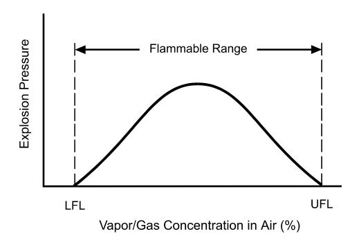
In popular jargon, a vapor/air mixture below the lower flammable limit is too "lean" to burn or explode, and a mixture above the upper flammable limit is too "rich" to burn or explode. The LFL is also known as the **lower explosive limit (LEL)**. The UFL is also referred to as the **upper explosive limit (UEL)**. No attempt is made to differentiate between the terms *flammable* and *explosive* as applied to the lower and upper limits of flammability.
