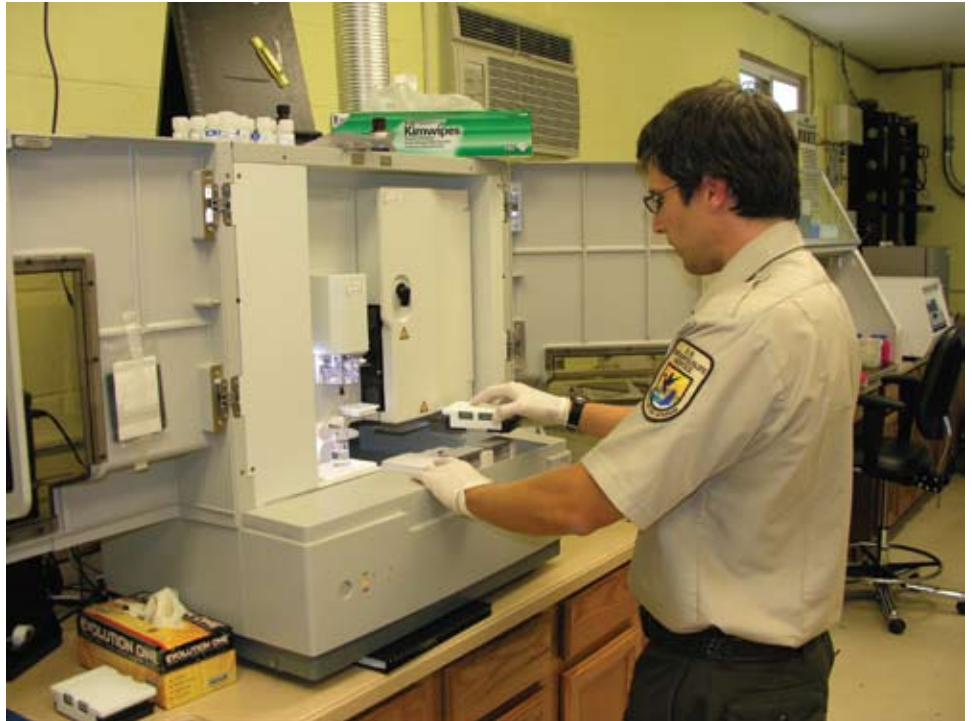
Dr. Greg Moyer loads Atlantic sturgeon DNA samples on an Applied Biosystem 3130 genotype analyzer.
