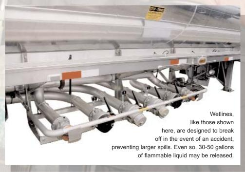
prevent spillage from the tank. Wetlines that don't contain flammable liquid may still contain flammable vapors, and responders should avoid potential ignition sources during the initial response.
