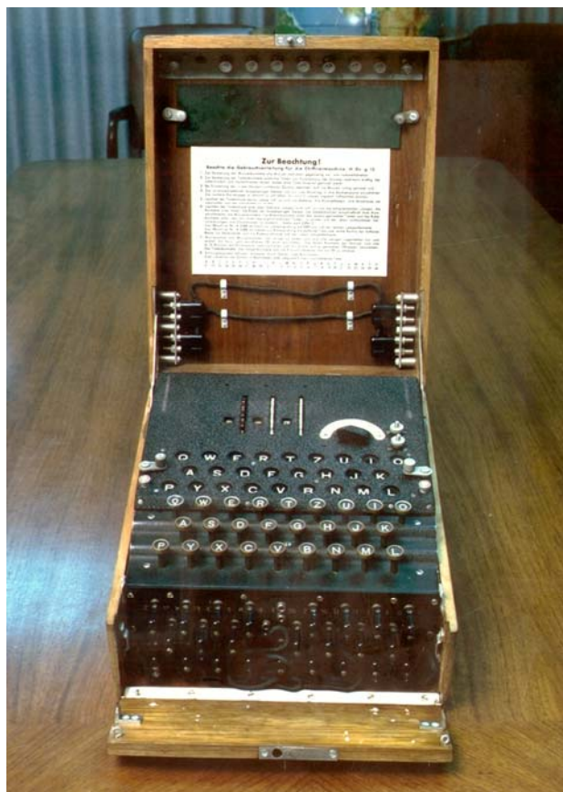
The Enigma was a portable cipher machine used to encrypt and decrypt secret messages
